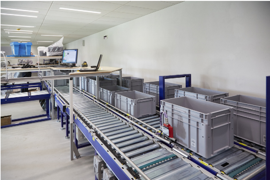
A work place for picking books form storage boxes and putting them back into the boxes.
